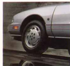
Available traction control helps maintain traction when accelerating on slippery road surfaces by detecting wheel spin during zero—30 mph acceleration and automatically correcting tire slippage.
