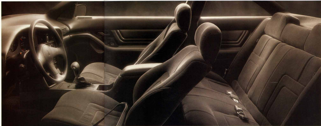
The Opti-Ride front bucket seats with adjustable driver-side lumbar support incorporate a unique seat suspension with an elastomeric mat stretched over the seat frame. The result is a front seat that will both conform to your body and remain supportive over time.
