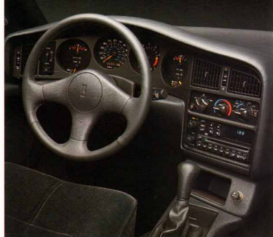
Left: The wraparound dash features full analog instrumentation. The steering column stalk controls include a one-step "flash-to-pass" feature and a wiper/washer switch that actuates a washer built into the wiper arm itself to help avoid freeze-up.
