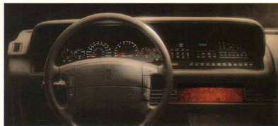
Driver-oriented analog instrumentation includes tachometer, and oil pressure, coolant temperature and voltmeter gauges.
